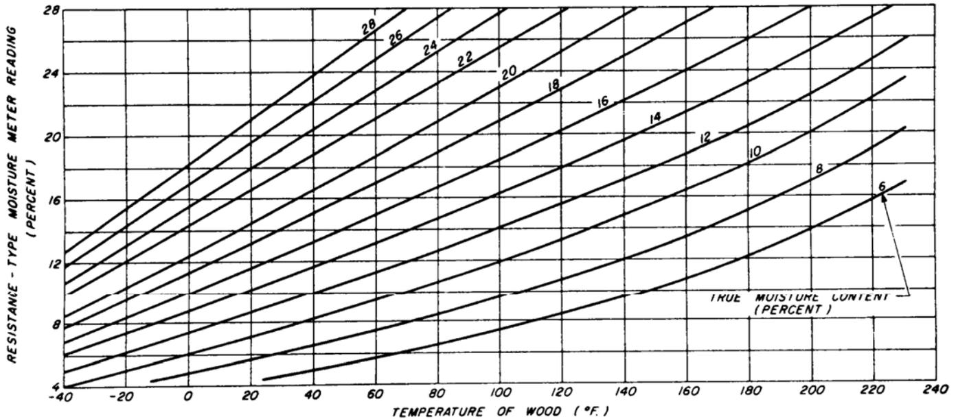
*Temperature corrections for use with resistance type moisture meters (James, 1988)*
