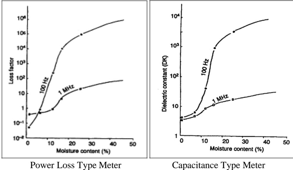
**Examples of (A) relationship between power-loss factor and MC% and (B) relationship between dielectric constant and MC%. (James, 1988).**
